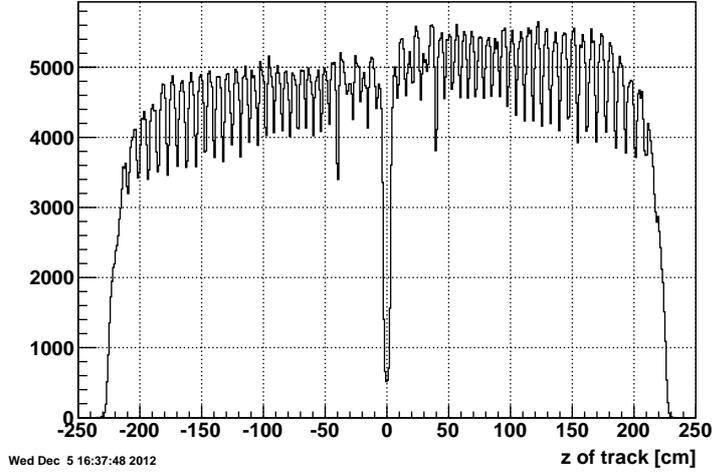
**Figure 3.** Projection of Fig. 2 over the horizontal axis ( $z$  coordinate of the track at intercept with the middle of the TOF detector ( $R=214.4\text{cm}$ )). The first 31 modules per tray are clearly visible. Module 32 is only seen as change of slope on the rapidly falling counts at the edge to the TOF detector.
