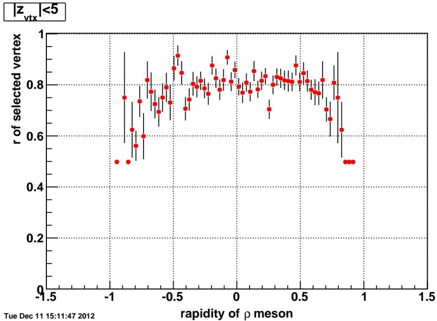
**Figure 15.** Average value of the ratio  $r$  of selected two track vertices as function of the rapidity of the  $\rho$  mesons candidates reconstructed in them. The distribution of  $z$  coordinate of those vertices is narrow:  $|z_{vtx}| < 5$  cm. in it.
