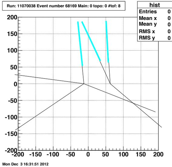
**Figure 10.** The yz projection of global tracks associated with a TOF hit are displayed in cyan color. The black lines show primary tracks in the event. This event has two vertices, both have tracks extrapolating to a TOF live cell, the value of the ratio  $r$  for both vertices is high and they will be included in the analysis separately.
