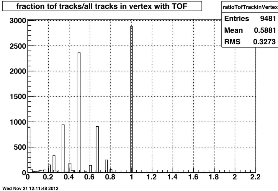
**Figure 7.** Ratio of number of tracks that extrapolate to a TOF hit over the number of all tracks in that particular vertex which extrapolate to the TOF z acceptance.
