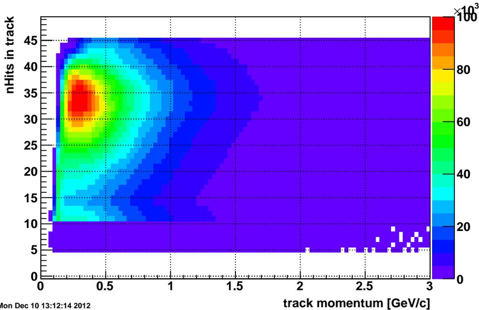
**Figure 6.** Same as Fig. 5 but this time the tracks are primaries from selected vertices ( $r \geq 0.02$ ), they intercept the geometrical acceptance of the TOF detector. Tracks with low momentum and number of hits below 14 tend to be related to particles spiralling inside the TPC active volume.
