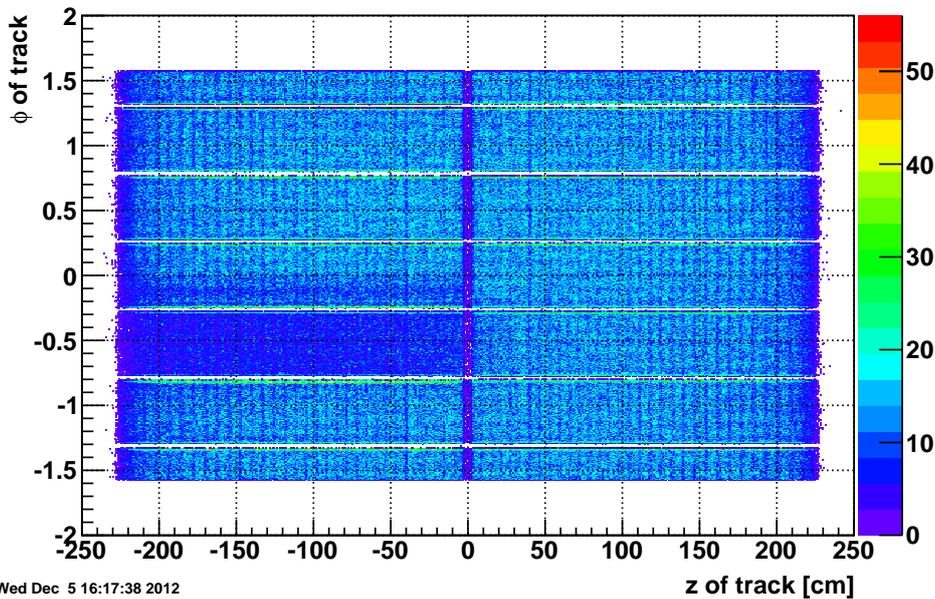
Figure 2. This figure shows the impact of charged particles on the nominal middle of the TOF detector. The vertical shows the azimuthal angle at the end point of the track that extrapolates to a live TOF cell, the horizontal axis shows the z coordinate of the intersection of the same tracks and a cylinder ( $R=214.4$  cm) that defines the nominal middle of the TOF detector.
