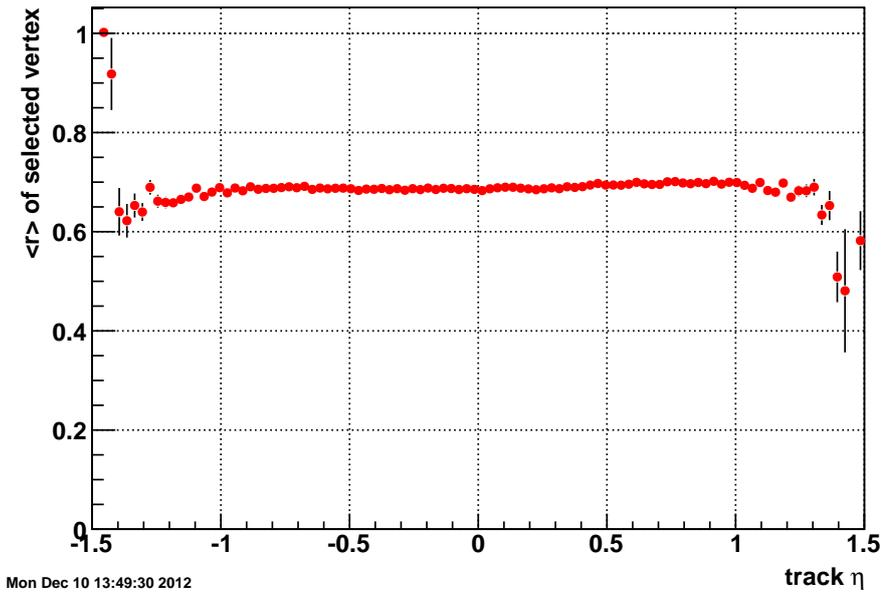
**Figure 13.** Average value of the ratio  $r$  of selected vertices as function of the pseudo-rapidity of the tracks originating from it. Vertices with  $R \leq 0.02$  are excluded from the sample.
