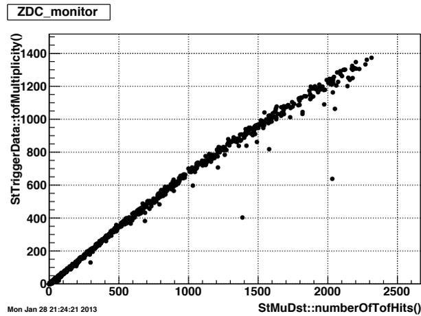
**Figure 17.** The number of TOF hits as seen by the trigger system (read from StTriggerData) versus the number of actual hits in the TOF detector (read from StMuDst). The correlation is filled with ZDC\_Monitor triggered events.
