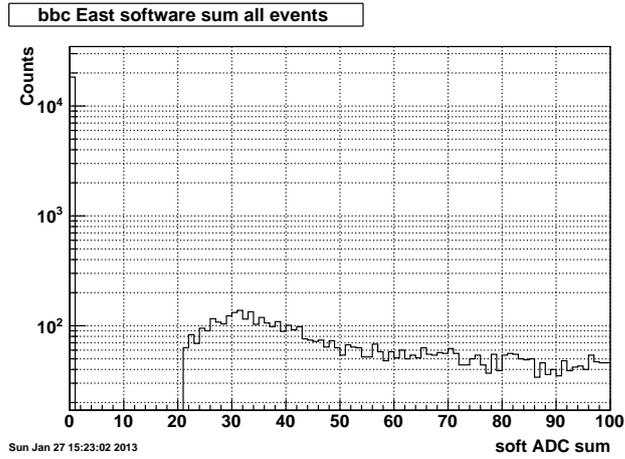
**Figure 10.** This distribution shows the offline sum of ADCs from small PMTs on the East BBC. In order to be included in the sum a PMT must have a signal corresponding to an ADC above channel 20. A cut imposed on this software sum at channel 50 defines the BBC veto in the UPC\_Main trigger.
