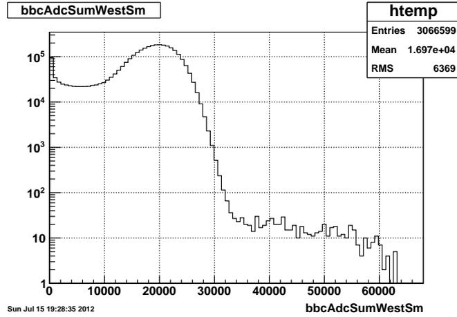
**Figure 6.** Same sum of ADCs as Fig. 3 but this time for the small BBC tubes on the West side.
