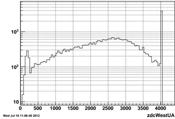
**Figure 13.** Same as Fig. 11 but filled with the sum of ADC from the ZDC West calorimeter for all events.
