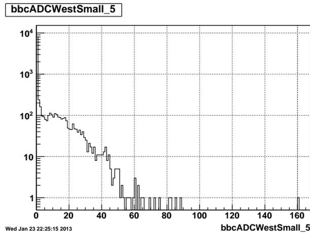
**Figure 7.** ADC distribution recorded for the small BBC tube number 5 on the west side for events that fired the UPC\_Main trigger.
