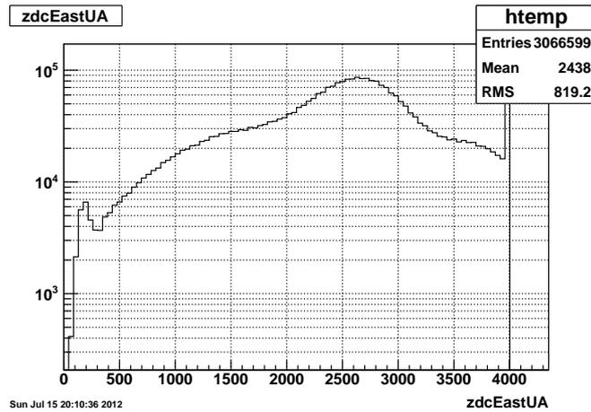
**Figure 11.** Unattenuated ADC sum for the East zdc calorimeters for all events collected. The single neutron peak is present at low ADC values and the signal saturates at channel 4000.
