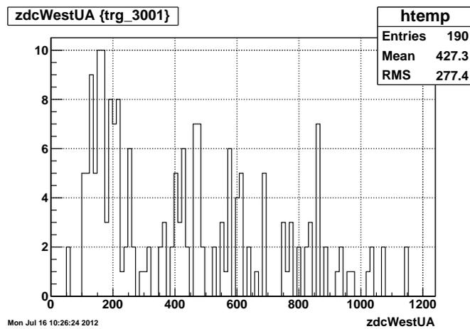
**Figure 14.** Unattenuated sum of ADCs for the West ZDC for events that satisfy the UPC\_Main trigger.
