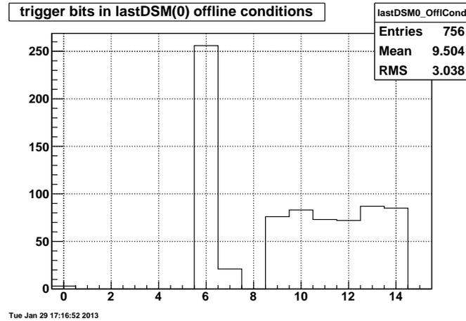
**Figure 21.** The first trigger word (lastDSM0) which carries TOF information related to the UPC\_Main trigger in bits 5 and 6. The histogram is filled with events that satisfy the offline conditions. All events that satisfy the offline cuts have bit 6 set.
