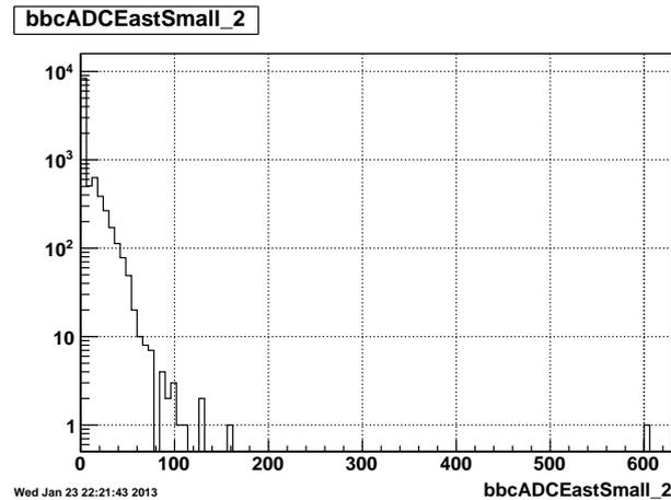
**Figure 4.** The ADCs recorded in the small BBC photomultiplier number 2 on the East side for events that fired the UPC\_Main trigger.
