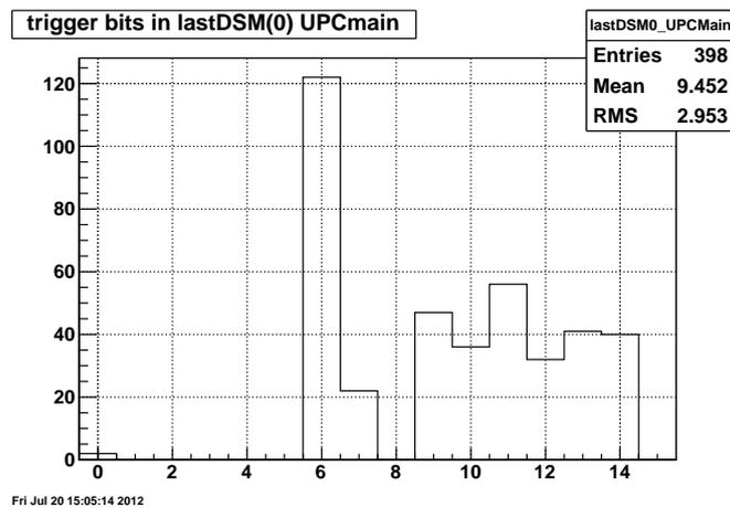
**Figure 19.** The first trigger word showing the bits for UPC\_Main firing events.
