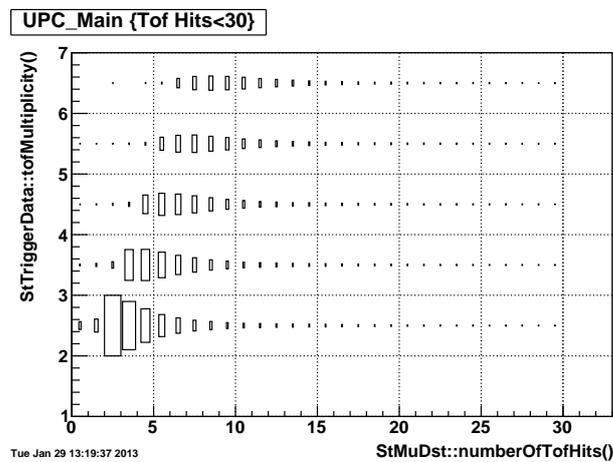
**Figure 18.** The number of TOF hits as seen by the trigger system (read from StTriggerData) versus the number of actual hits in the TOF detector (read from StMuDst). This correlation is filled with events triggered by UPC\_Main.
