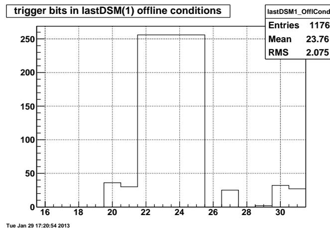
**Figure 22.** Second trigger word (lastDSM1), which carries BBC and ZDC information related to the UPC\_Main trigger, is filled with ZDC\_monitor events that satisfy the offline conditions. No entries are seen in bits 17 or 18 corresponding to the BBC vetoes on East and West sides respectively, and all the ZDC bits have 256 entries
