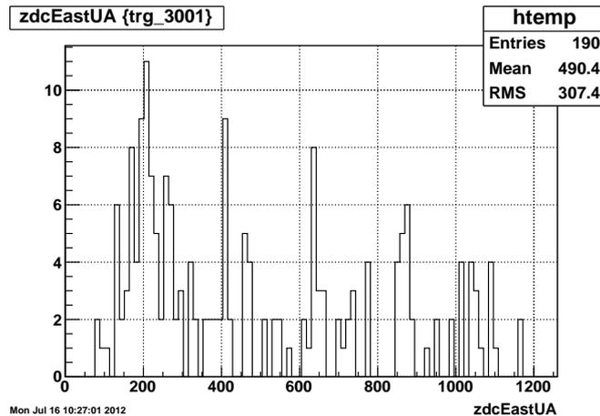
**Figure 12.** Unattenuated ADC sum for the East ZDC calorimeter for events that fired the UPC\_Main trigger.
