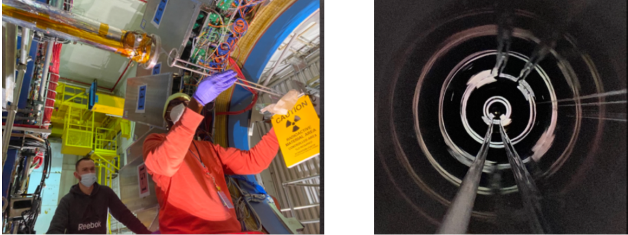
Figure 67: Left panel: Installation of the targets and holder on the East side of the STAR detector. Right Panel: A view down the beam pipe showing the three targets (C, Al, and Ni) installed at STAR.
